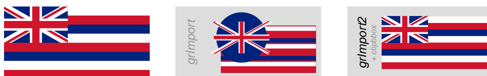
Figure 11: At left, the state flag of Hawaii as an SVG image (from Wikipedia). In the middle, the flag after importing and rendering with grImport , which does not import clipping information. At right, the flag after importing and rendering with grImport2 .
