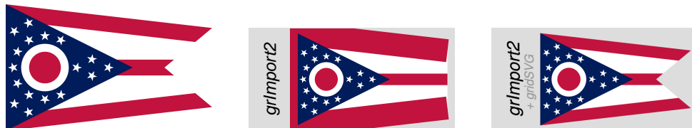
Figure 12: At left, the state flag of Ohio as an SVG image (from Wikipedia). In the middle, the flag after importing and rendering with grImport2 on a standard R graphics device; the non-rectangular clipping information in this flag cannot be rendered correctly on a standard graphics device. At right, the flag after importing with grImport2 and rendering with gridSVG .
