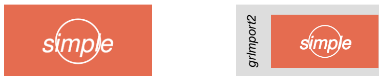
Figure 5: On the left is a simple SVG test image consisting of only paths and text. On the right is the result of converting the image to Cairo SVG using grConvert then importing and rendering the image using grImport2 .
