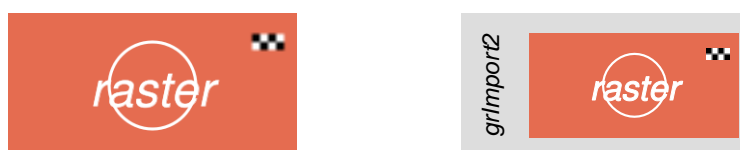
Figure 6: On the left is an SVG test image that contains a raster element. On the right is the result of converting the image to Cairo SVG using grConvert then importing and rendering the image using grImport2 . The important point is that the raster element is retained during the import process.
