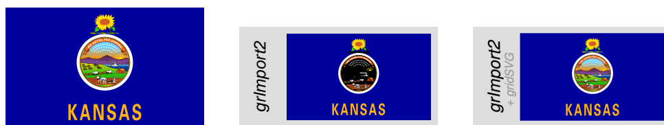
Figure 10: At left, the state flag of Kansas as an SVG image (from Wikipedia). In the middle, the flag after importing and rendering with grImport2 on a standard R graphics device; the standard device cannot render the gradient fills, which results in black regions on the flag. At right, the flag after importing with grImport2 and rendering with gridSVG .
