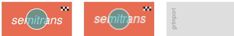
Figure 3: On the left is a test image that is in an SVG format and that contains a semitransparent fill. In the middle is the result of converting the original image to a PostScript format with ImageMagick, which results in rasterisation of the image. On the right is the result of importing and rendering the converted image with grImport , which does not work very well because grImport does not import raster elements.
