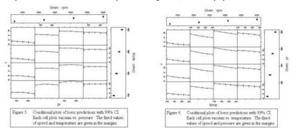
predicted vacuum using sets of 4-by-4 conditioning plots. The vertical bars are 99% confidence limit for the fit. The vacuum vs. speed plots (Figure 4), indicates quadratic dependence, a linear term (*i.e.*
