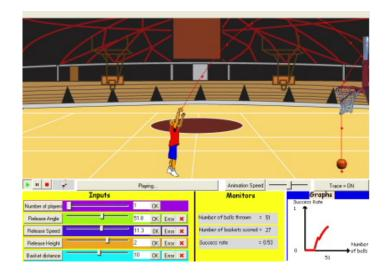
Figure 1. The player has successfully thrown the ball into the basket. The release angle, speed, height and distance can all be varied using the sliders or by entering the data directly. Once the play button has been pressed, the player continues to throw with the given parameters until the pause or stop button is pressed. The trace of the ball can be switched off. Feedback is shown in the Monitors and Graphs panes.
