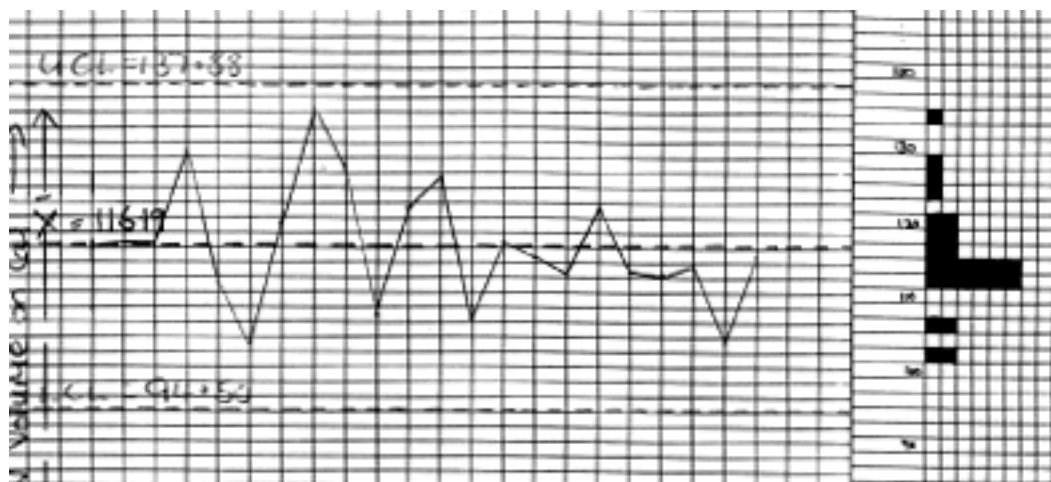
Figure 1. Part of an SPC chart on airtightness of cars
