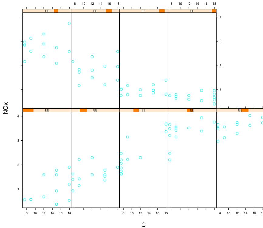
**Figure 5.** Scatterplots show NO<sub>x</sub> emissions as a function of compression ratio for various values of equivalence ratio.
