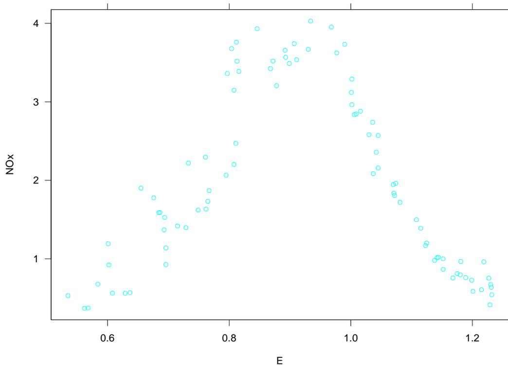
**Figure 1.** A simple scatterplot of the engine data, showing `NOx` emissions as a function of equivalence ratio.
