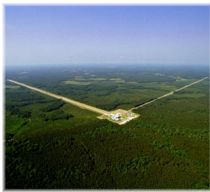
Layout sketch and actual interferometer with 4-km arms.
