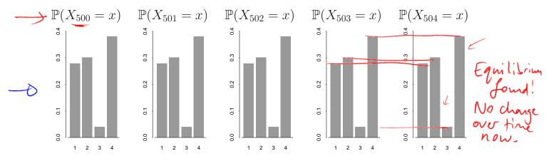
The distribution has reached a steady state: it **does not change** between  $t=500,501,\ldots,504$ . The chain has reached equilibrium of its own accord.
