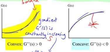
G''(s) > 0 means that the gradient of G is constantly increasing for OKSKI.
