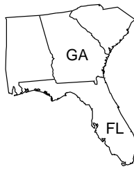
Figure 5.13: A map of the south-eastern United States produced using the Albers equal area projection.
