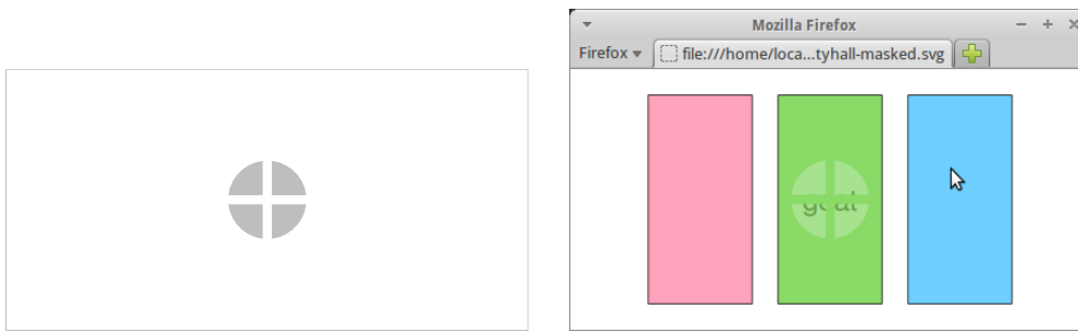
Figure 6: Using a mask on an image. The picture on the left shows a white cross on top of a grey circle on a white background. This is used as a mask on the rectangles in the Monty Hall image on the right. The effect is to create a semitransparent window in the middle door (through which we can glimpse the word “goat”).
