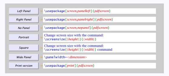
Figure 1: Different types of panel positioning
