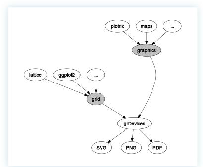
The 'grid' package provides an ALTERNATIVE graphics system to the 'graphics' package ("base" graphics). Many packages define plotting functions based on 'graphics', but there are some important ones based on 'grid', such as 'lattice' and 'ggplot2'.
