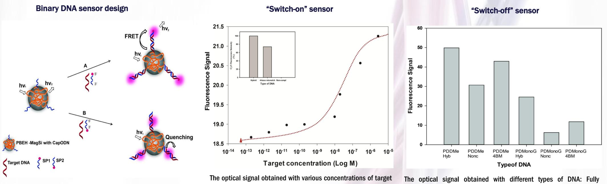
Design of our novel binary DNA sensor with either "switch-on"(A) or "switch-off") (B) optical readout.<sup>1</sup>
